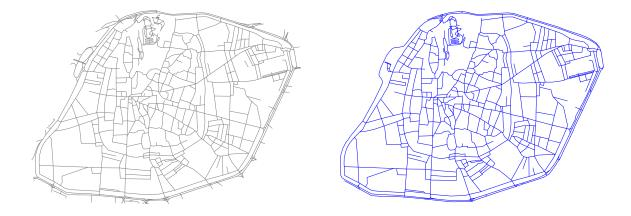
8. If you don't perform this step of quick export, you will get the result as the left one shows that the arcs are not chopped into segments at each junction. The needed result is represented in the right one and all the arcs are cut into segments.
